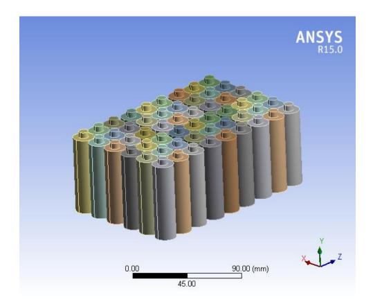
The thermal analysis is performed in the workbench ansys software, which is to be determined how much heat flux will be generated in the total and also directional heat flux and also temperatures of maximum.
